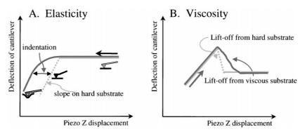
Fig. 7. Appearance of force curves when the sample indents under the tip (A) and when the jump-off-contact is slowed down due to viscosity of the sample (B).
